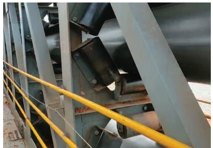
Pipe conveyor cross-section (similar to Yubei). CREDIT: CONVEYOR DYNAMICS
