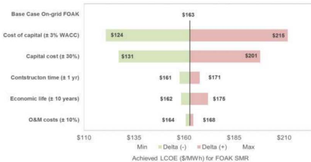
Figure 14 Sensitivity of LCOE for on grid SMRs to key parameters (source: SMR Roadmap)
