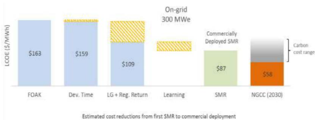
Figure 15 Estimated cost reductions from first SMR to commercial deployment (Source: SMR Roadmap)
